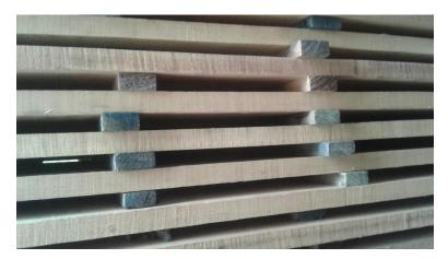
The 50 mm boards and boards of other dimensions were transported to Scion in Rotorua for air or slower kiln-drying. Several logs were sent to JNL in Kaitaia for a peeling trial, which went off smoothly.
