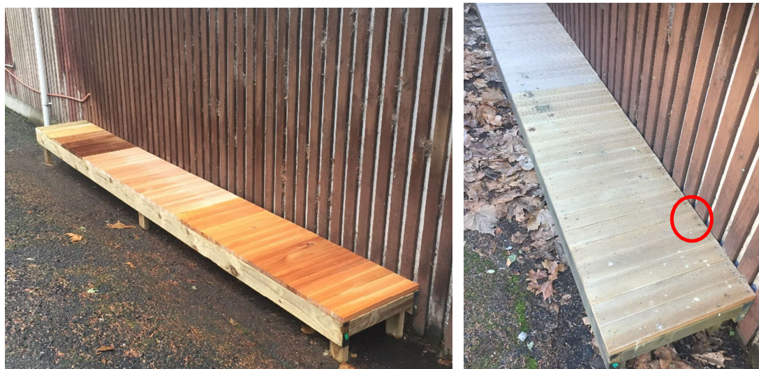
Illustration 5 (L to R): Decking trial on installation and after 12 months exposure (circle with staining near screws)
