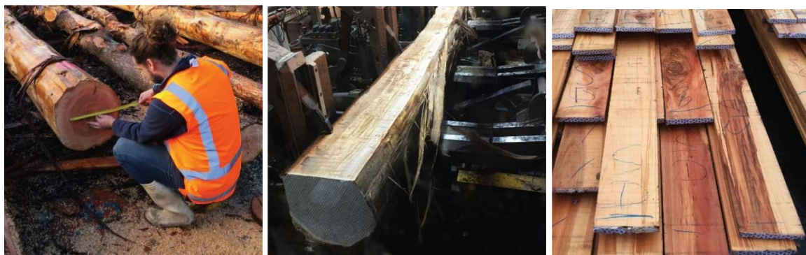
Illustration 2 (L to R): Assessing heartwood content at Toi Ohomai training mill site; Logs going through sawmill; Tōtara boards after grading prior to drying (June 2018, Photos: Greg Steward and John Lee)
